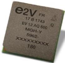
It has a 7GHz analog bandwidth and many nice features like the Cross Point Switch, which transforms the ADC from a 1 to 4 channels, the Sampling Delay Adjust, and easy multi-chip synchronization feature. It has successfully passed radiation testing up to 150kRad and is already Space-proven.
